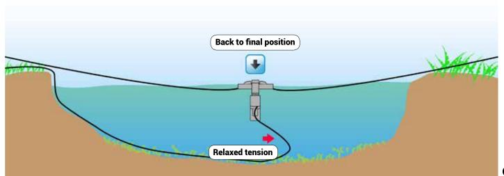
4. Hold the position of the unit in the water by tying the mooring lines securely to the mooring stakes.
