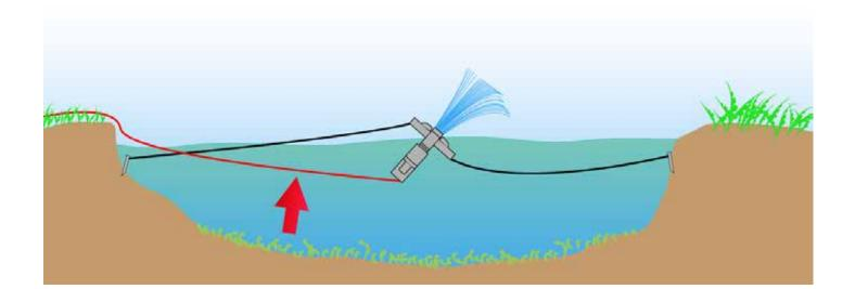
3. Anchor line too tight (if anchored to the bottom):
