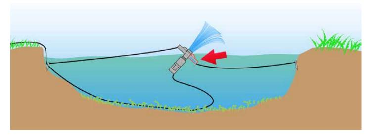
5. Possible blockage in the nozzle tips: If water is spurting out with higher or lower pressure on one side due to a blockage or damage to the nozzle, it can cause the fountain to tip. Please check the nozzle tips to ensure they are clear and undamaged.
