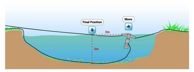
3. Bring the unit back to the final position. There should be enough slack on the electric cable to allow it to hang down without tension on the unit causing it to tilt the spray pattern. Drive in mooring stakes to secure mooring lines
