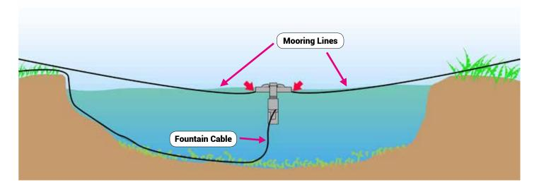
2. Pull the unit past its final location by a distance at least equal to the depth of the dam at the desired final location.
