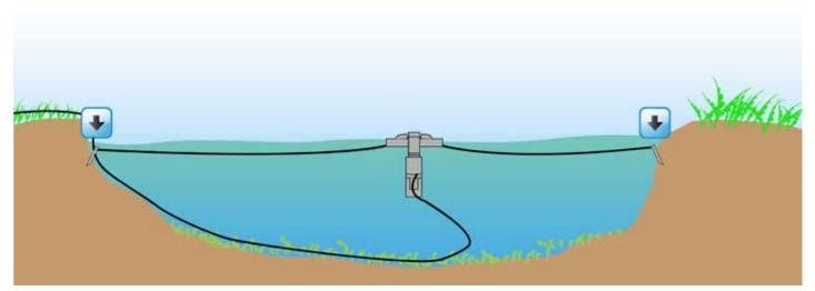
5. Motor torque causes the unit to try to rotate if the mooring lines are not tight. Upon start-up, watch to make sure the unit cannot rotate more than 1/3 of a turn. If it is allowed to rotate, the electric cable can pull around the unit very tightly and cause damage.
