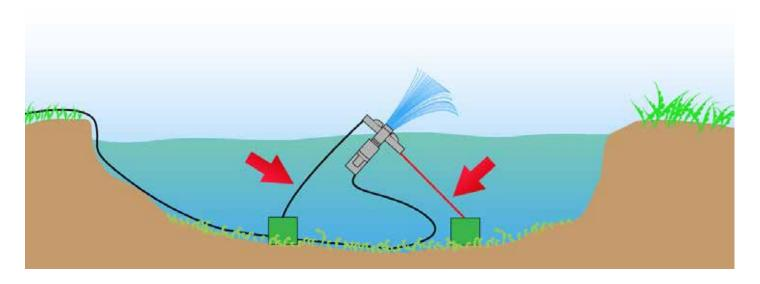
4. Water in the float: A crack or leak in the float can cause it to take on water and tilt to one side. Inspect the float for any damage where water could be leaking in.
