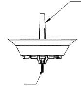
Finally secure the Center (.6)Nozzle Tip to the Nozzle base using 2x screws
