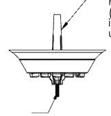
Finally secure the Center (.6)Nozzle Tip with the plug inserted to the Nozzle base
