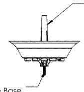
Finally secure the Center (.6)Nozzle Tip to the Nozzle base using 2x screws
