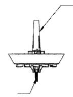
Finally secure the Center (.6)Nozzle Tip with the plug inserted to the Nozzle base using 2x screws
