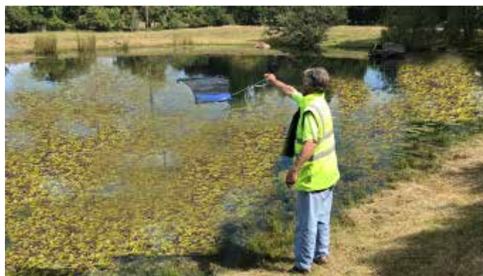
STEP 2 - Hold the very end of cord, toss out the skimmer.
