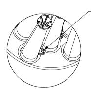
Install 12 x Flow Controls to holes 1-12 on the underside of the Nozzle Base with 1 screw each
