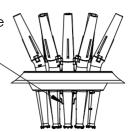
Finally attach a .6 Nozzle tip to the center of the Nozzle Base using 2 screws
