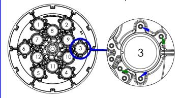
Install 6x **Group 1** Nozzles on holes 7-12 Install 6x **Group 2** Nozzles on holes 1-6
