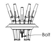
Secure the Nozzle Base to the Unit using the bolt that goes through the center hole
