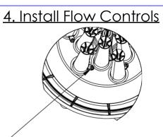
Install 12x Flow Control to holes 1-12 on the underside of the Nozzle Base with 1 screw each
