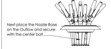
Finally attach the .5 Nozzle Tip to the center of the Nozzle Base using 2 screws
