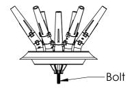
Secure the Nozzle Base to the Unit using the bolt that goes through the center hole
