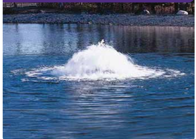
2 HP Floating Surface Aeration Mixer
